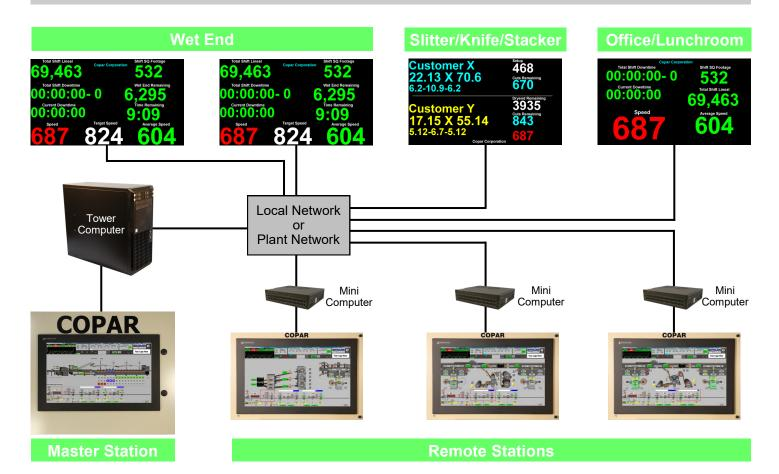
The Master Station and Remote Stations allow the operators to perform routine tasks.
