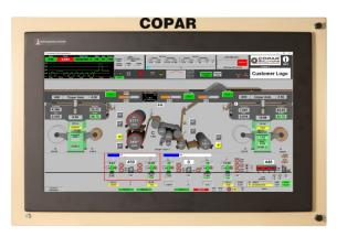
Because of the compact design, the panels can be mounted to a wall, a support beam, above an existing operator console, or can be installed with an optional Copar floor mounting stand. Remotes are typically located near each singlefacer, and one near the stacked doublebacker preheaters.
